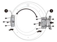
5 Remove the door catch **6** from the appliance frame by removing 2 screws and then
