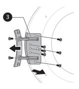
Remove the 3 screws from the door latch assembly which is fixed between the door and the hinge assembly, and then remove the screw which is fixed on the door hook.
