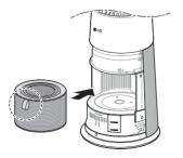
Insert the fixing part on both sides at the bottom of the cover into the fixing groove in the bottom of the product, and then close the cover.
