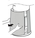
Remove dust surrounding the Aero Series V Filter from the ultra-fine filter with a vacuum cleaner or soft brush.
