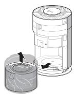
4 Install the filter in the appliance with the side where the filter handle is attached facing up.
